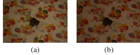
Figure 2. Color changes due to difference in camera sensitivity. (a) Image taken with Canon D600 under tungsten lamp illumination. (b) Image taken with Nikon D5100 under the same illumination.
