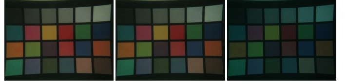
Figure 6: Change in observed colors with distance from water surface.
