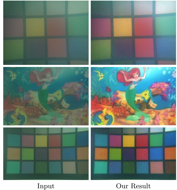
Figure 9: Experiments on images taken at same reference depth but with higher turbidity.
